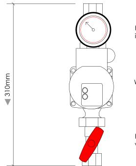
Flanged ball valve with in-handle thermometer
